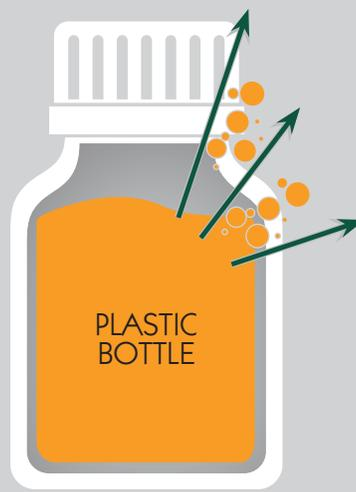
**Transpiration** refers to the passage of water vapor through the walls of a container and/or evaporation from the container opening. Transpiration results in an increase in the concentration of the CR/RM.
